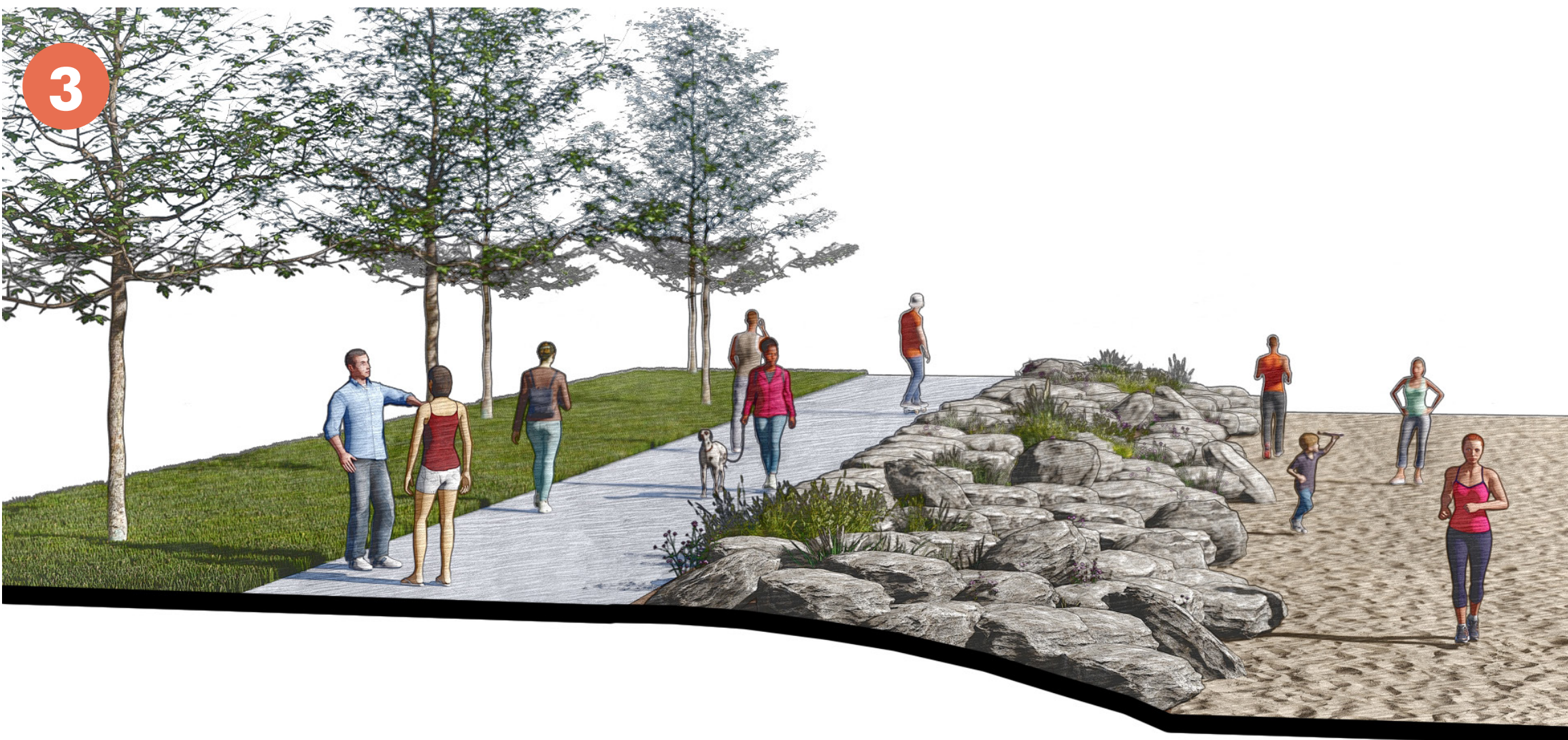
A LIVING SHORELINE is a protected, stabilized coastal edge made of natural materials such as plants, sand, or rock.
