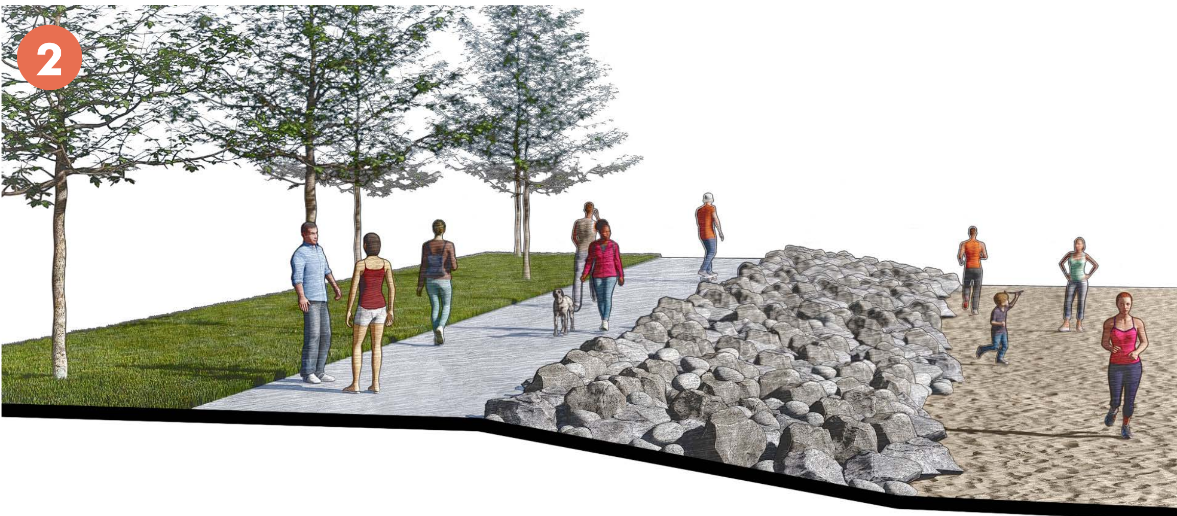
RIPRAP is an engineered shoreline protection strategy that consists of large rocks along the shoreline to protect the area that is subject to wave action induced erosion.
